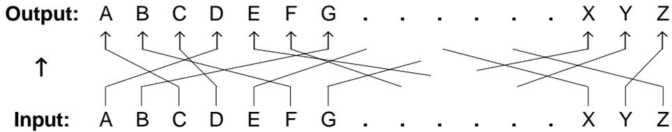
so that when key A was pressed the output was D, when B was pressed the output was G, and so on. In fact, our message would be put into cipher as it was being keyed in. It would be a simple cipher since every plain text letter would be enciphered in exactly the same way. But if the wiring could be readjusted quickly you would have the basis of a real ciphering machine.
